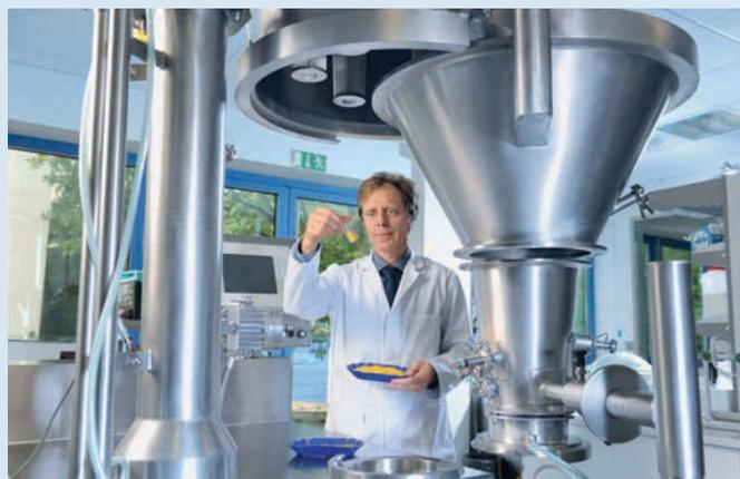
density and a low specific surface area; this makes them especially suitable for the subsequent application of functional layers by coating. Spray granulation permits very precise adjustment of parameters such as particle size, residual moisture and bulk volume. The method is used, for example, when the objective is to create a homogeneous, dustless product with a high bulk weight.
