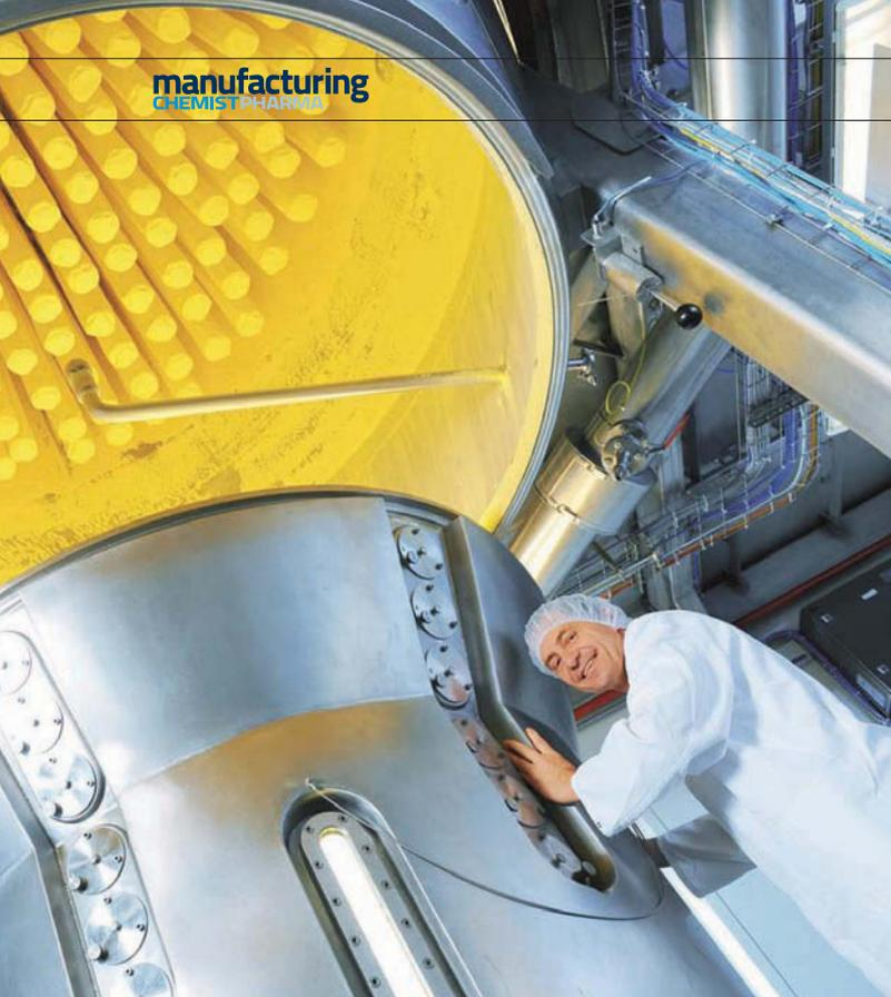
surface of the particles and simultaneous drying causes the powder particles to adhere to each other and form free-flowing agglomerates. Bridges of solid matter form between the individual particles in the course of drying, thus causing the agglomerates to grow. This improves the physical handling of the goods, since the agglomerates produced in this way contain far less dust, have better tableting properties, are readily soluble and also easier to dose because of their enhanced flowability.
